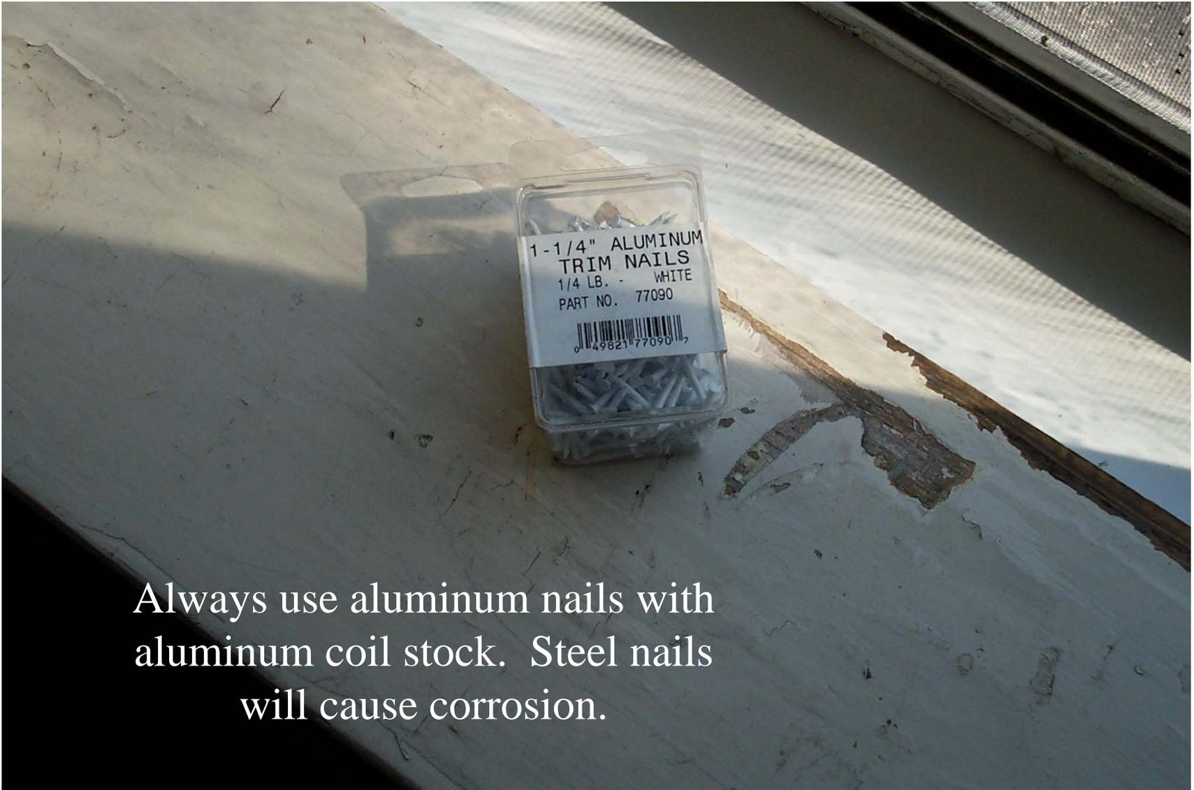
Always use aluminum nails with aluminum coil stock. Steel nails will cause corrosion.
